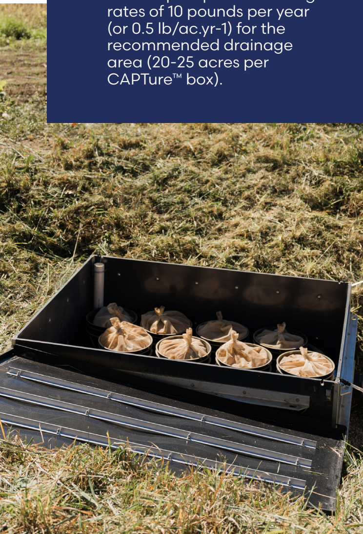
Figure 5. CAPTURE™ box interior with filter vessels and filter media bags.
