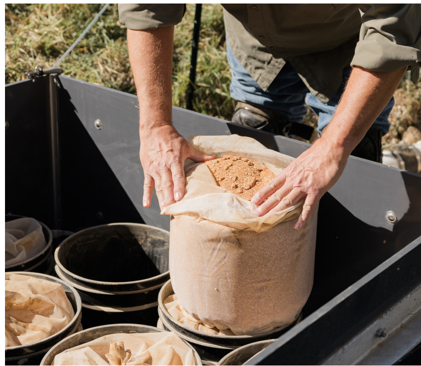
Figure 5. CAPTURE™ box interior with filter vessels and filter media bags.
